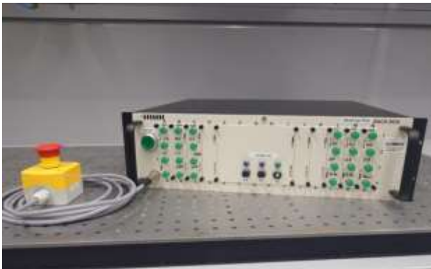
Fig. 2 Multi-Cap project: The amplifier can serve up to 12 data channels in a single fiber strand.
