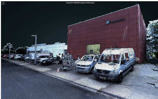
Fig. 2 In the visual representation, the point clouds are colored using camera images. The end result is a virtual 3D environment that combines vividness with precision geometric information. Users can move around freely in the virtual scenery.
