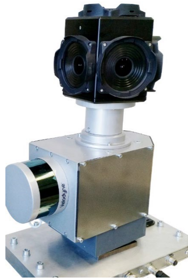
Fig. 1 The LiDAR laser is attached to a rotating turntable. The laser scans an area of 16 vertical sections, or “slices,” per second. In total, the device emits 1.3 million laser pulses per second. This data is then used to produce a 3D point cloud of the environment.
