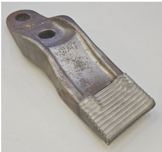
Fig. 2 Mining tools like this excavator bucket tooth are subject to extreme wear. Ultra-accurate AI-assisted laser material deposition is used to perform repairs quickly and cost-effectively right on the machine.
