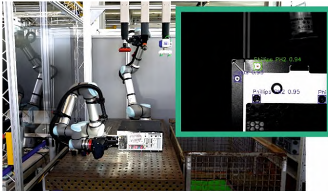
Fig. 2 The robot locating and approaching the screws on the computer housing.
