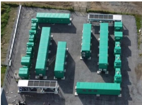
Fig. 2: The test bench for the offshore wind turbines is capable of testing even very large turbines up to an output of 28 megavolt-amperes (MVA).
