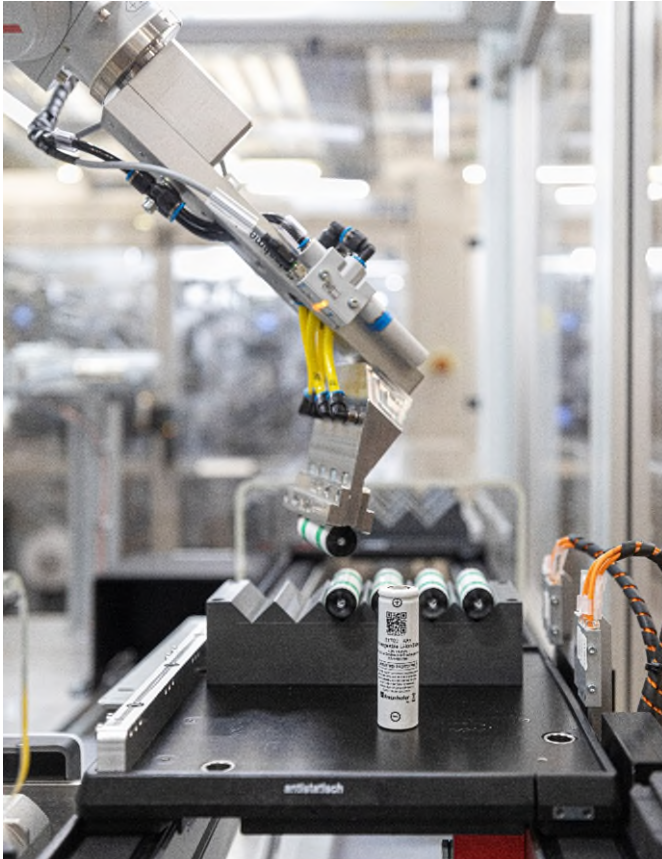
Fig. 1 Jelly rolls and cylindrical battery cell produced at Fraunhofer IPA (21700 round cell in tabless continuous design)
