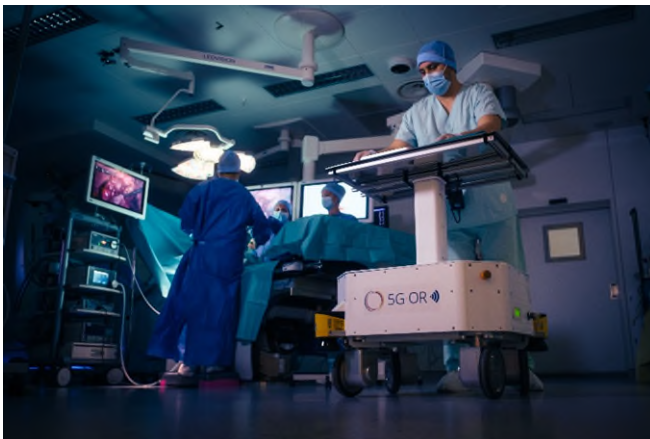
Fig. 1 The mobile robotic platform developed by Reutlingen University together with Fraunhofer IPA in the experimental OR in Strasbourg enables the autonomous transport of medical material and instruments.
