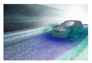
Fig. 2 The cloud of numerical points that is used can adapt flexibly to moving geometries. This saves time when simulating complex processes such as driving through water.
