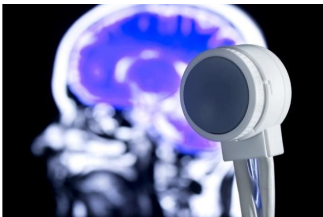
Picture 1: The 3D matrix ultrasound transducer for transcranial neurostimulation can stimulate specific points deep inside the brain with precision targeting.
