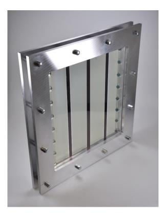
Individual module of a standalone tandem PEC reactor.
