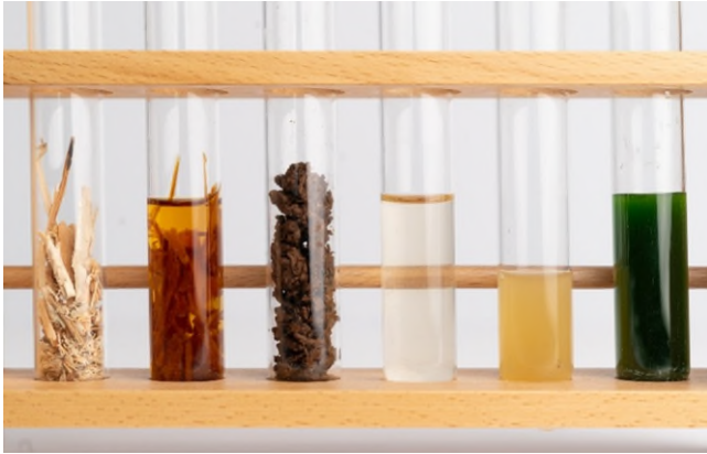
Fig. 2 From left: Untreated old wood, wood in pulping solution, cellulose fibers (after boiling and washing), sugar solution from cellulose fibers, anaerobic hydrogen producers (bacteria), microalgae
