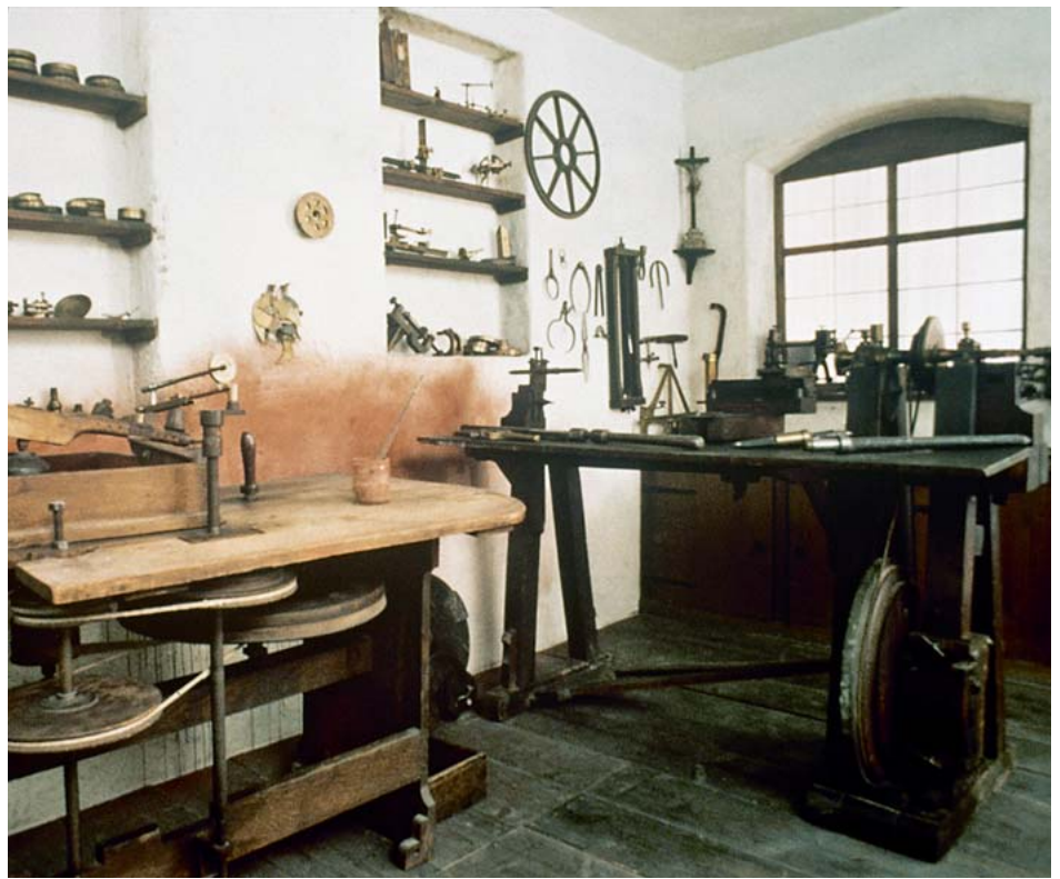
The workbenches in Fraunhofer's workshop used to grind and polish lenses.
