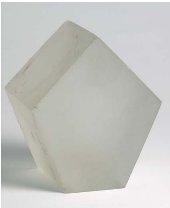
Fraunhofer carried out several series of systematic tests to develop new types of optical glass. The picture shows a pentaprism produced by him.
