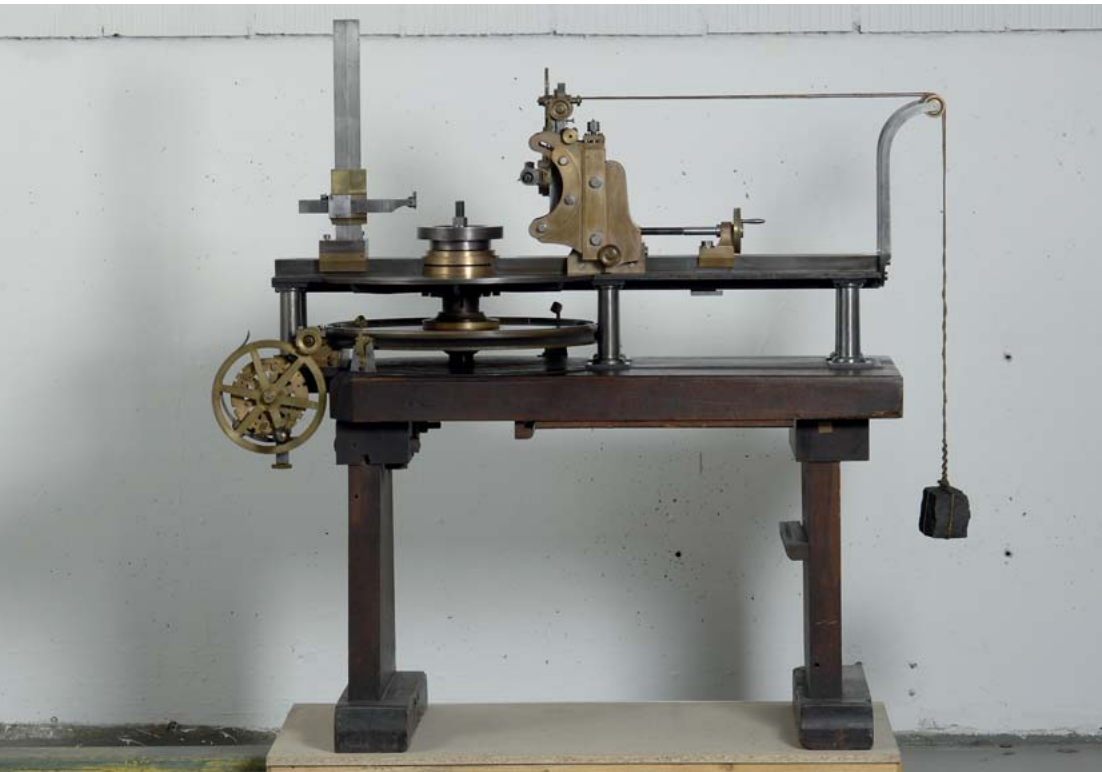
Gear milling machine from Fraunhofer's glassworks.
