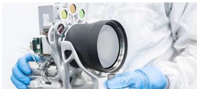
Infrared imager in the ERNST small satellite
