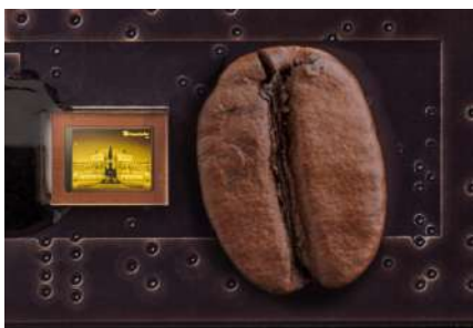
OLED microdisplay with the world's smallest pixels
