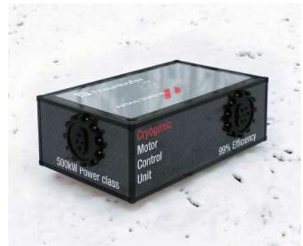
Cryogenic drive inverter for electric drives in aviation
