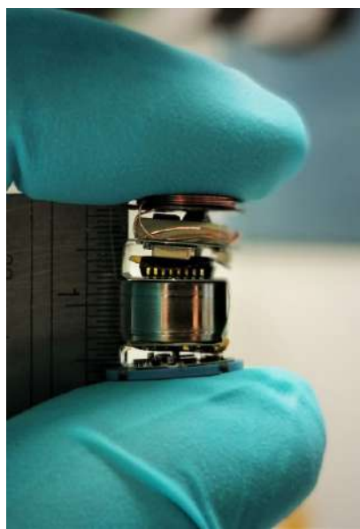
Extremely miniaturized spectroscopy capsule for a wide range of diagnostic options
