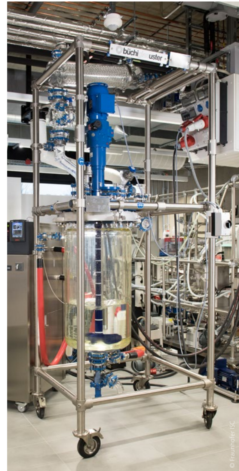
100 liter synthesis reactor for the upscaling of catalyst materials to industrial pilot plant scale at Fraunhofer ISC, coupled with various in-line analysis technologies
