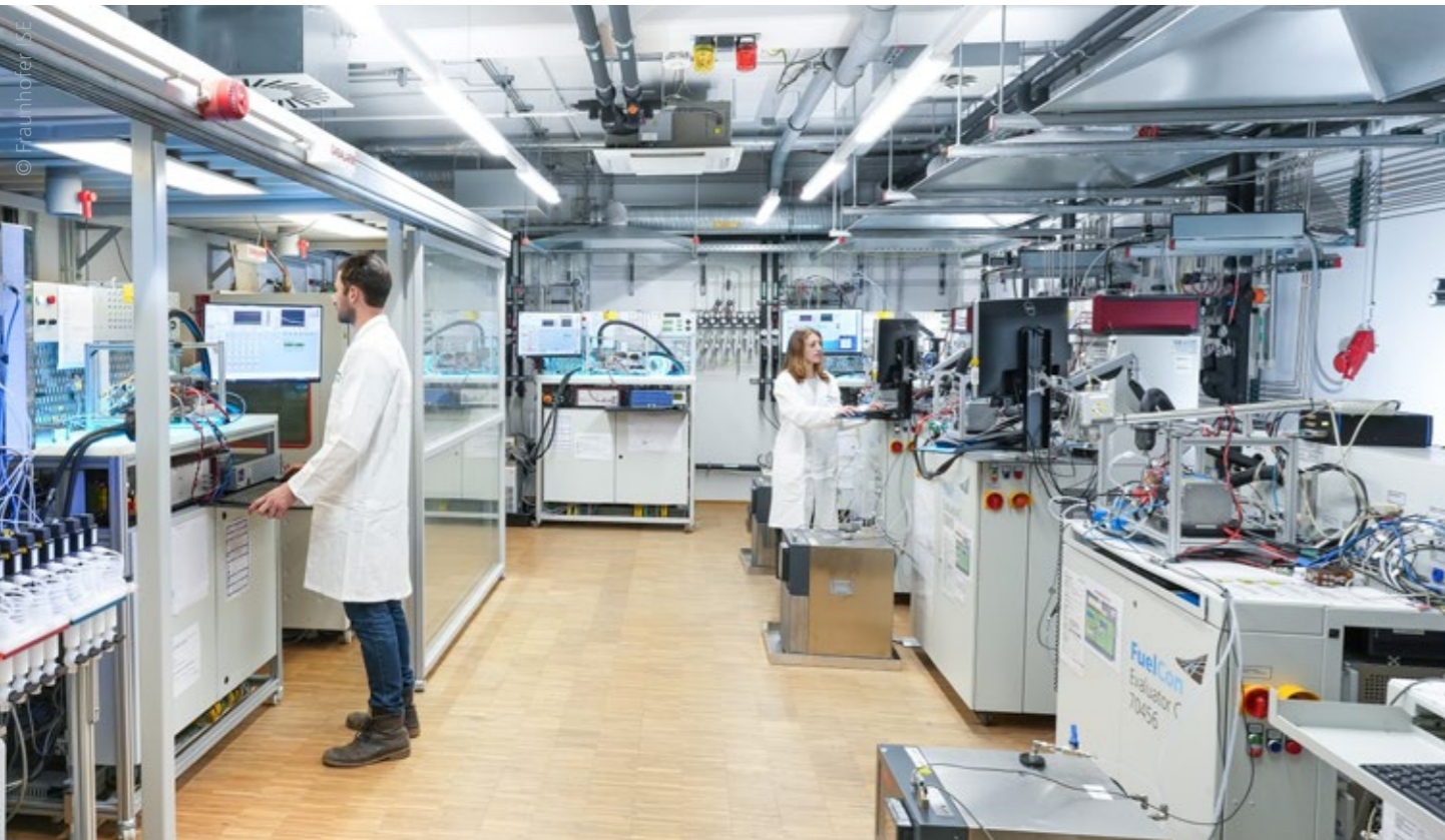
Test rigs for the electrochemical characterization of membrane electrode units for PEM fuel cells at Fraunhofer ISE.
