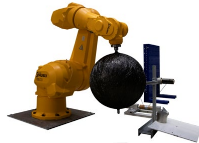
Production of an isotensoid spherical tank in the KuWaTa project
