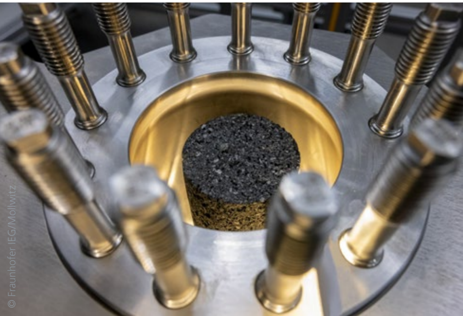
Porous rock sample placed in Fraunhofer IEG's H_2 autoclave for tests under pressures of up to 50 MPa and temperatures of up to 200°C, as part of an experimental investigation into rock-fluid interaction within potential storage horizons for hydrogen.
