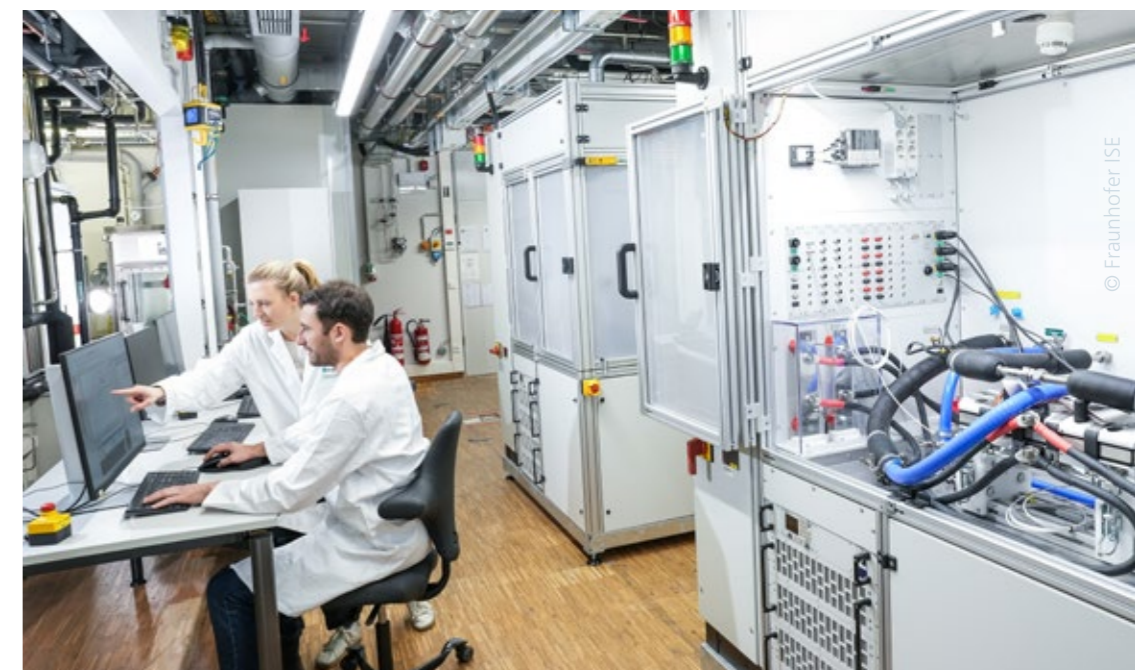
Test rigs to characterize fuel cell short stacks for mobility applications, at Fraunhofer ISE.
