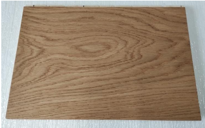
Fig. 1 The protein/additive combination, applied to the surface of oak flooring with an oil-based topcoat.
