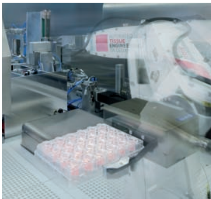
A fully automated system is used to process and cultivate the skin samples. © Rafael Krötz/ Fraunhofer IGB
